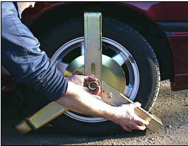
8. Still holding up nut with left hand, pull the right wheel clamp arm in tightly to tyre.
