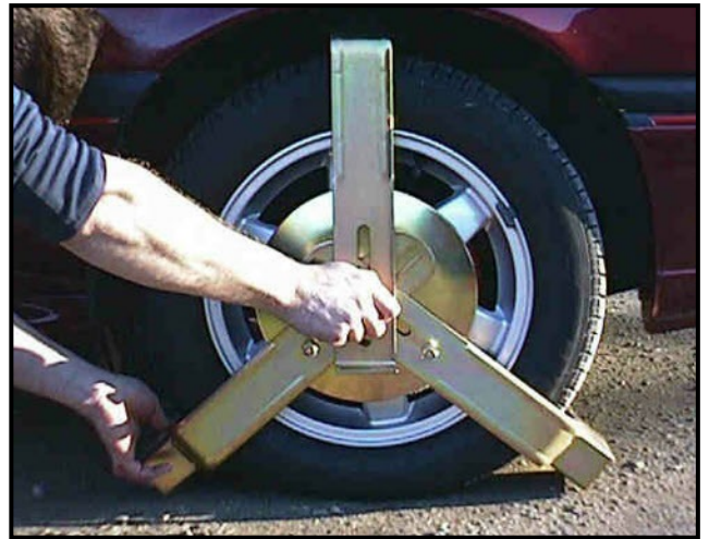
9. At this point hold up nut with right hand and pull left wheel clamp arm in tightly to tyre. Now hand tighten nut.
