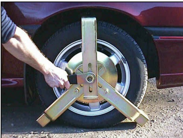
10. Using spanner provided tighten nut in a clockwise direction until it locks up solid. NB. When removing clamp reverse steps 10 to 6.
